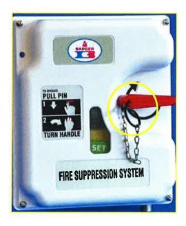
To manually engage the fire suppression system pull the pin shown in the image to the right and circled in yellow and turn red handle to the down position.
